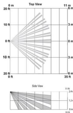
Figure 7: High Sensitivity Setting
